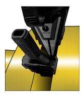
Ensure the full width of the selected Safety Block step is fully inserted before gradually retracting the tool until the flange load has been applied to them.
