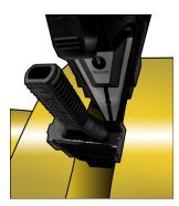
To use the next smallest step, actuate the wedges to around 75% prior to inserting back into the joint. Place the tool in the gap and actuate enough to relieve the load on the Safety Blocks. In this way the flange joint can be progressively closed.
